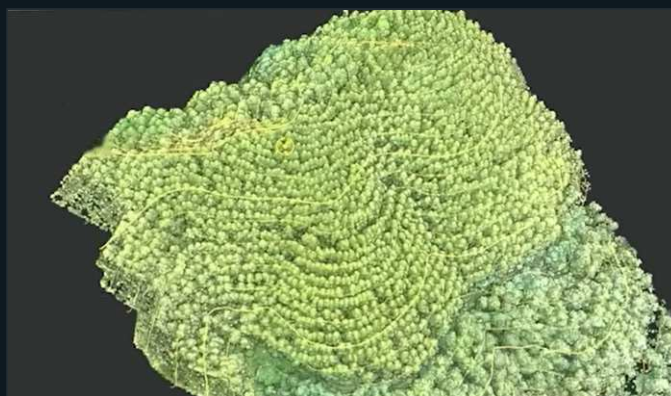
CANOPY SURFACE WITH DERIVED CONTOURS
