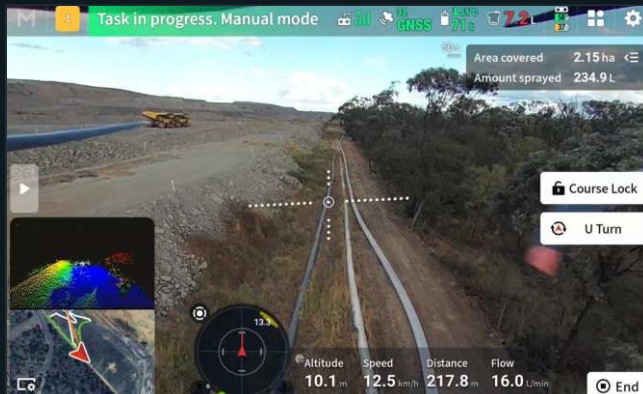
VARIABLE-RATE APPLICATION ALONG A MINE SERVICES CORRIDOR – LIVE COVERAGE AND VOLUME ON THE OPERATOR DISPLAY
